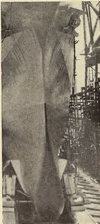
The sharp edge at the water line of our modern freighters, combined with a bulbous nose below the water line, serve to control the formation of the waves, thus saving power to put into speed.
